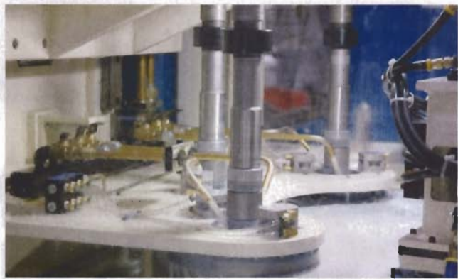
▲ Production honing with automatic tool wear compensation is available on this three-station Nagel ECO-40PVT single pass honing system.
