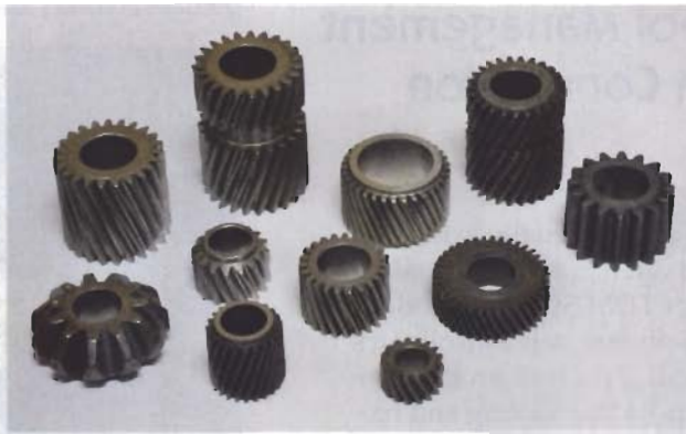
◀ Shown are some single pass honing application examples: connecting rod (left) and gears (right) made of powered metal and wrought steel.
