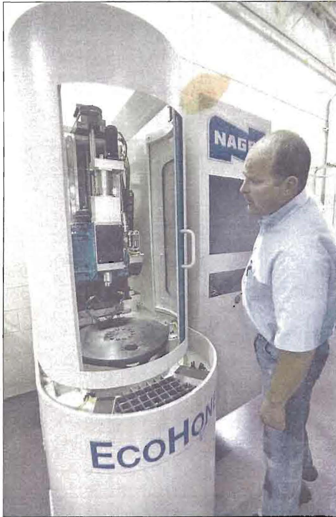
Assembly leader Mark Woods with a honing machine created for a tool show. The machine refines the shape and surface of parts.
